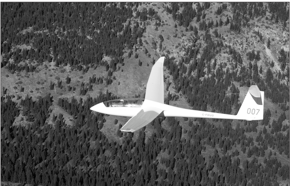
The high performance (L/D of 45 to 1) Duo Discus two-seat sailplane is used for cross-country training and passenger flights in Invermere, BC.
