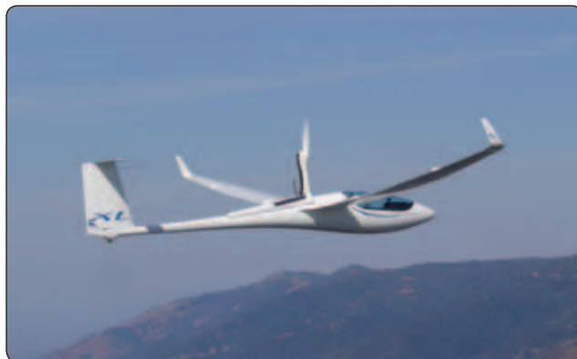
Figure 1-7. An ASH 26 E self-launching sailplane with the propeller extended.
