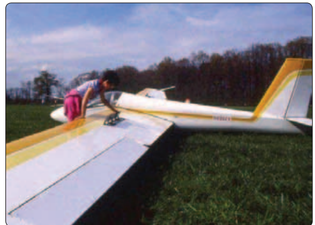
Figure 6-14. Positive control check of spoilers.
