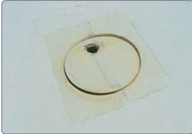
Figure 5-21. Water ballast tank vented filler cap.
