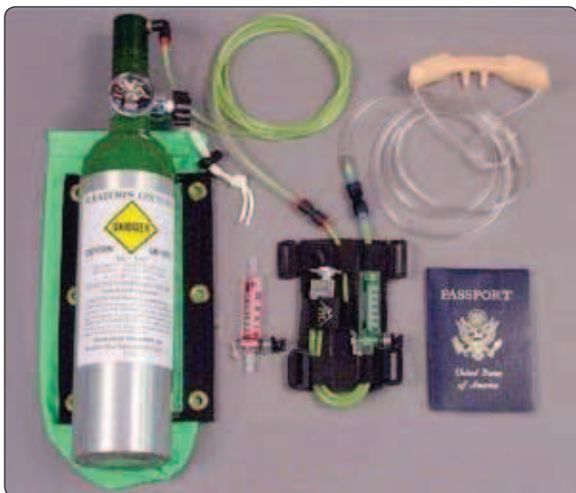
Figure 13-9. Continuous-flow oxygen system.
