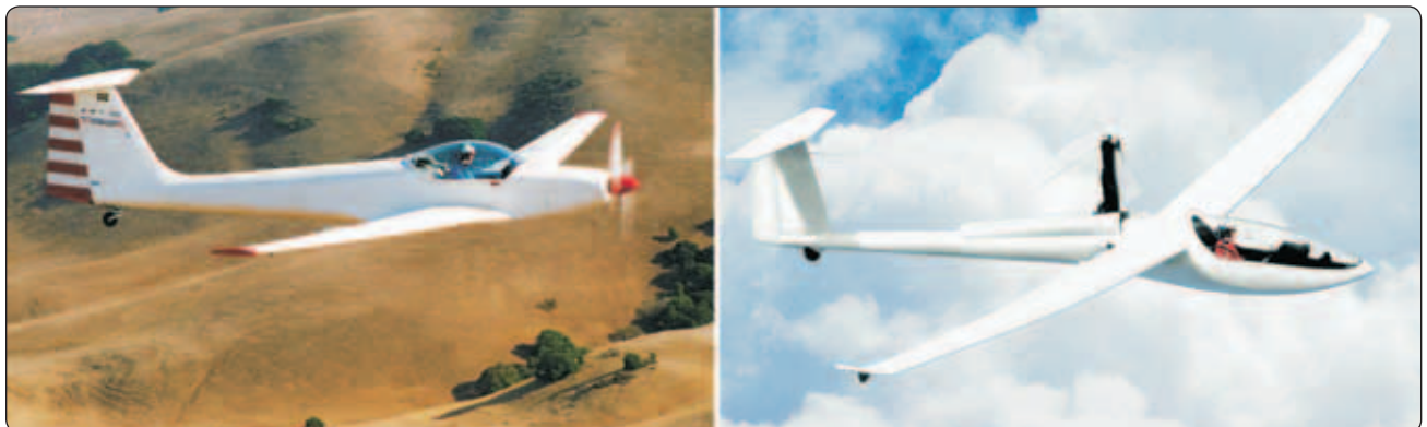
Figure 7-22. Types of self-launching gliders.
