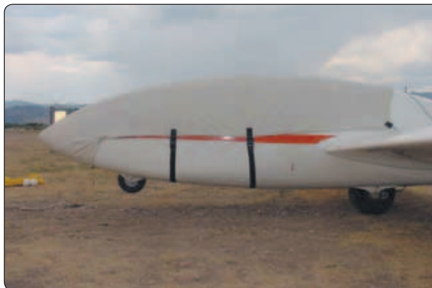
Figure 6-5. Protecting the canopy.
