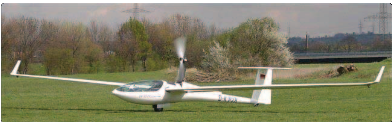
Figure 2-16. A DG-808B 18-meter high-performance glider in self-launch.
