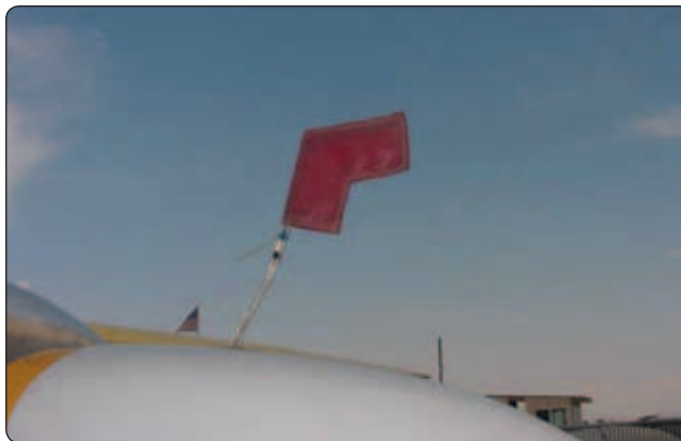
Figure 6-4. Protecting the pitot tube and total energy probe.
