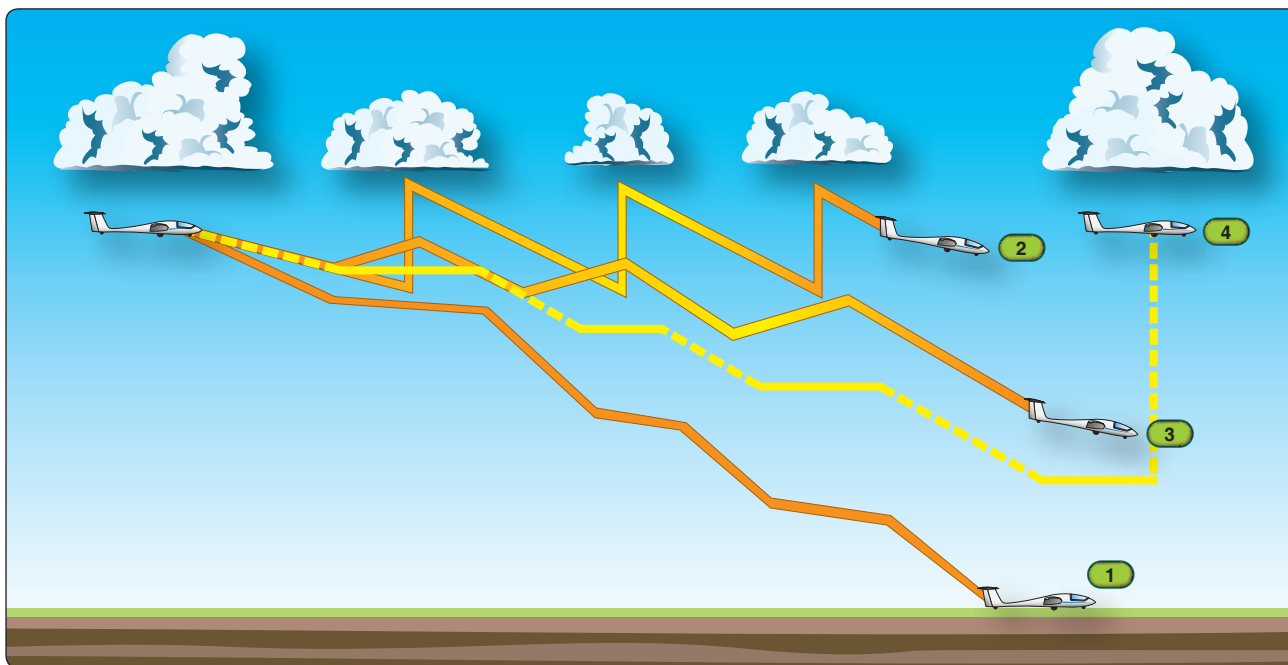
Figure 11-13. Example of glides achieved for different MacCready ring settings.
