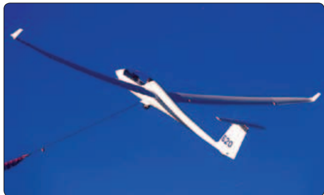
Figure 2-2. Schmepp-Hirth Ventus-2 glider with factory winglets installed.
